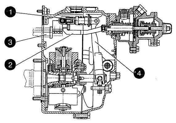
The temperature—dependent starting control—rod—travel regulation (TAS) is designed to prevent the cold—start control position being reached on hot starting and with the accelerator pedal fully depressed.
